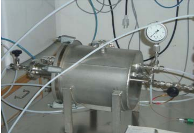
Picture 5.1.1.1. Small pressure chamber made of stainless steel
